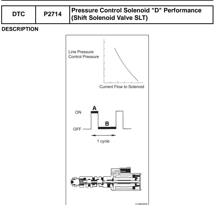
The linear solenoid valve (SLT) controls the transmission line pressure for smooth transmission operation based on signals from the throttle position sensor and the vehicle speed sensor. The ECM adjusts the duty ratio\* of the SLT solenoid valve output signal to control the hydraulic line pressure coming from the primary regulator valve. Appropriate line pressure assures smooth shifting with varying engine outputs. \*: The duty ratio is the ratio of the continuity to non-continuity in one cycle.
